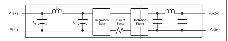
Figure D: Internal Input and Output Filter Diagram (component values listed in Electrical Characteristics section)
