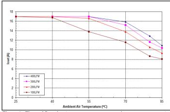
Figure 4: Thermal Derating (max output current vs. ambient air temperature) for encased converter with 0.7" heatsink, at airflow rates of 100 LFM through 400 LFM. Air flows across the converter from input to output (nominal input voltage).
