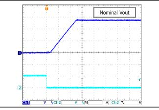
**Common Figure 1: Startup Waveform** (typical). Input voltage pre-applied, ON/ OFF Pin on Ch 2. Output voltage normalized.
