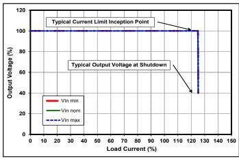
Common Figure 2: Output I-V Characteristics (output voltage vs. load current) showing typical current limit curves and converter shutdown points.
