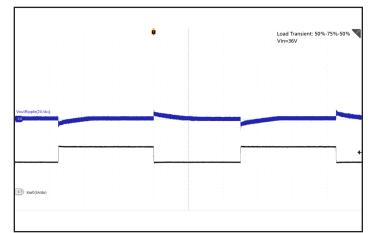
Figure 5: Output Voltage Response to Step-Change in Load Current (50 % -75 % -50% of Iout(max));  $dI/dt = 0.085A/\mu s$ .
