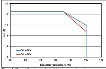
Figure 3: Thermal Derating maximum output current vs. baseplate temperature.
